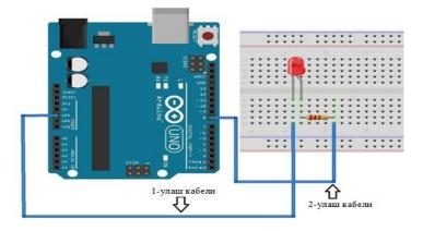
Figure 3: Connecting the blinking LED on the Arduino board
