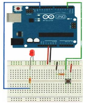
**Puc 5:** Wiring diagram for a LED controlled by a key
