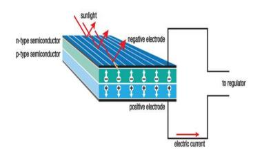
1-The process of generating electricity in a silicon solar cell.
