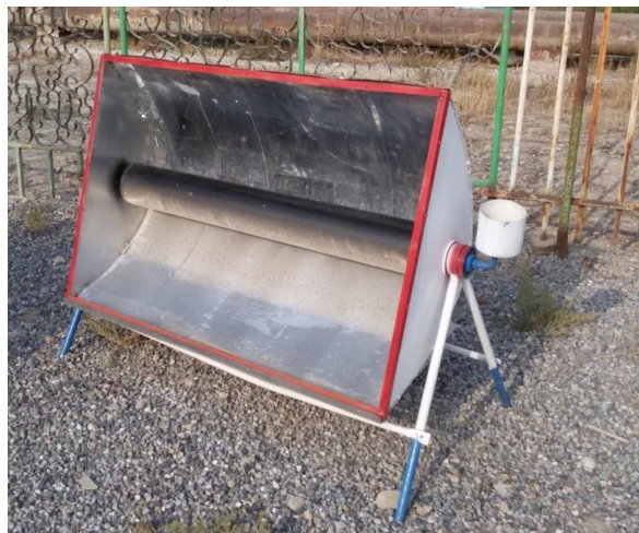
Figure 1. Construction scheme and general appearance of a parabolocylindrical solar water heater.
