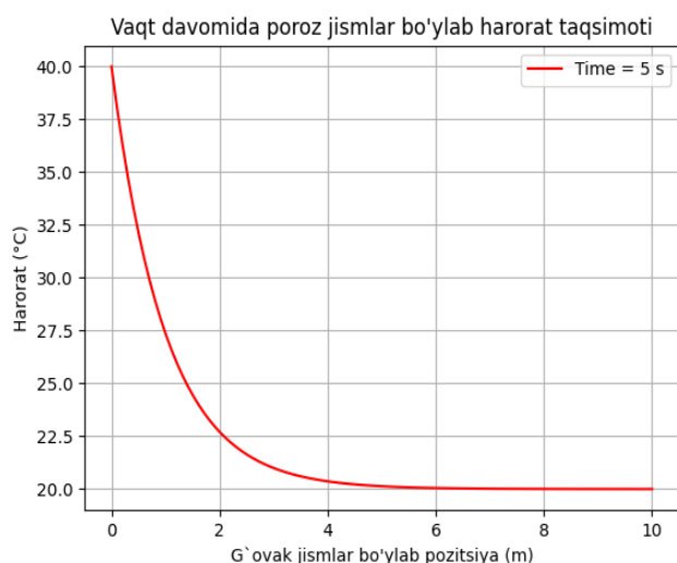
2-rasm. Vaqt davomida issiqlik o'zgarishi T_a = 20^{\circ}\text{C} , T(x, y, z, 0) = 40^{\circ}\text{C} .
