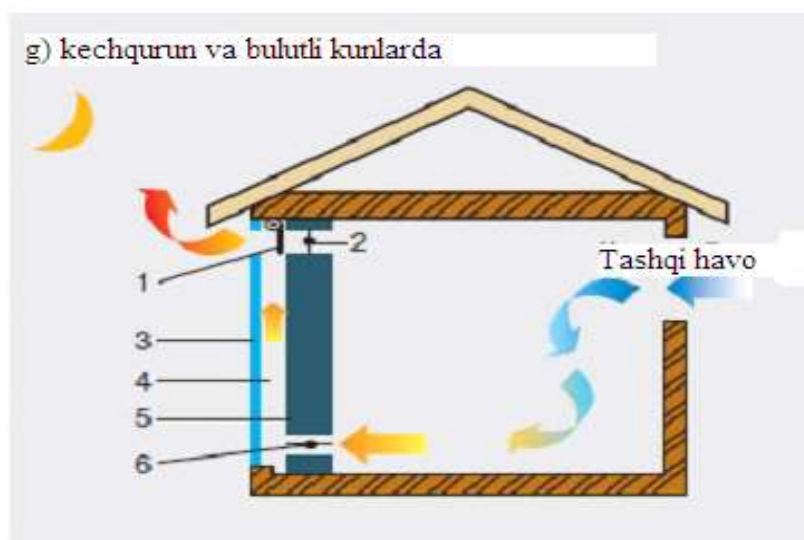
5g-rasm. g) Yoz mavsumi uchun. 1-parda, 2-yuqori klapan, 3-shisha to'siq, 4-havo qatlam, 5-massiv devor va 6-pastki klapan.
