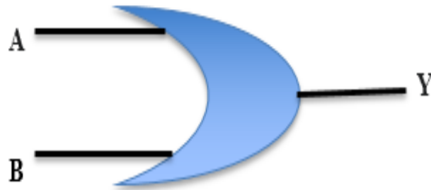
Figure 2: An OR gate logic circuit with two input digital signal and one output digital signal.
