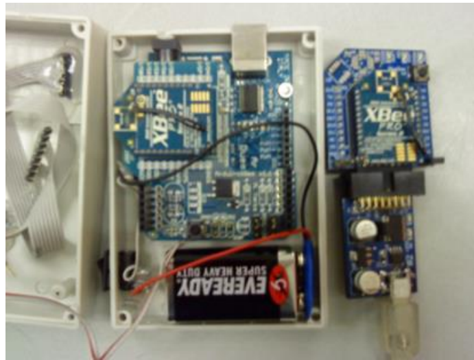
Figure 1: Xbee with Arduino (left) and BlueBee dongle (right)
