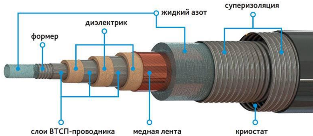
2-rasm. VTSP kabel qurilmasining tuzilishi.
