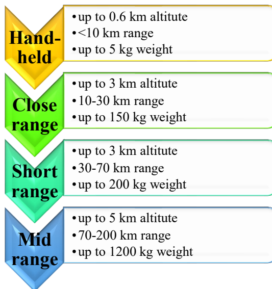
Fig. 2. UAV Classification by range
