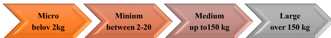
Fig. 1. UAV classification by Weight
