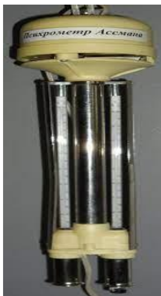
1-rasm. Assman psixrometri.
