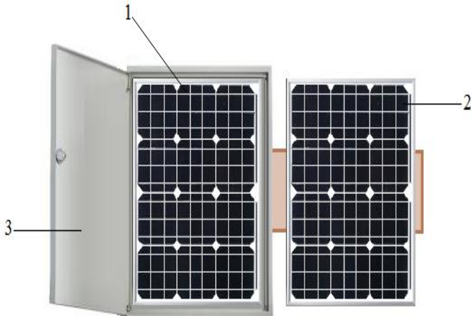
Figure 3. Setting up PVBs for the experiment 1 – PVB, the surface of which can be opened only at night, 2 – PVB, the surface of which is always open, 3 – cover
