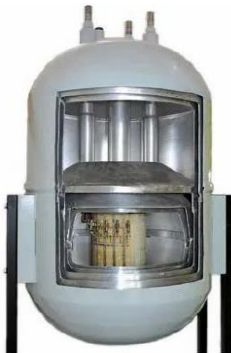
2.5-rasm. Matryoshka termos printsipli.
