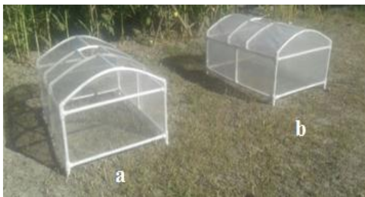
Fig. 1. Experimental devices covered with polyethylene film: a - ordinary polyethylene; b - functional ceramic composite polyethylene
