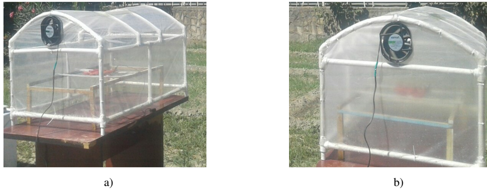
FIGURE 4. The appearance of solar dryers during the experiment: a) with a traditional ordinary polyethylene coating; b) solar dryer with functional ceramic composite polyethylene coating.
