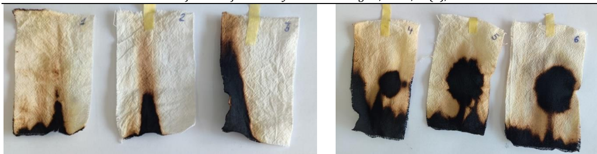
Fig. 13. Flame-retardancy test on cotton fabric samples
