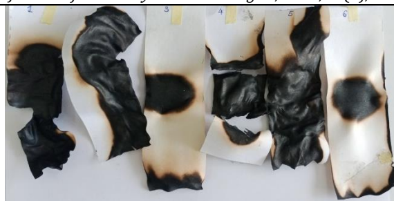
Fig. 11. Flame-retardancy test on paper samples
