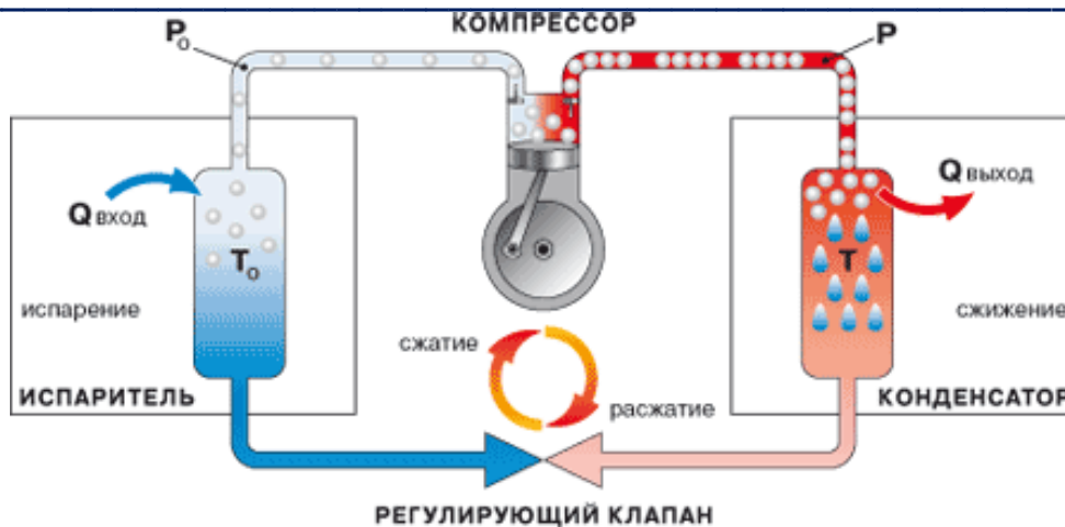
Fig. 3. Heat pump devices.
