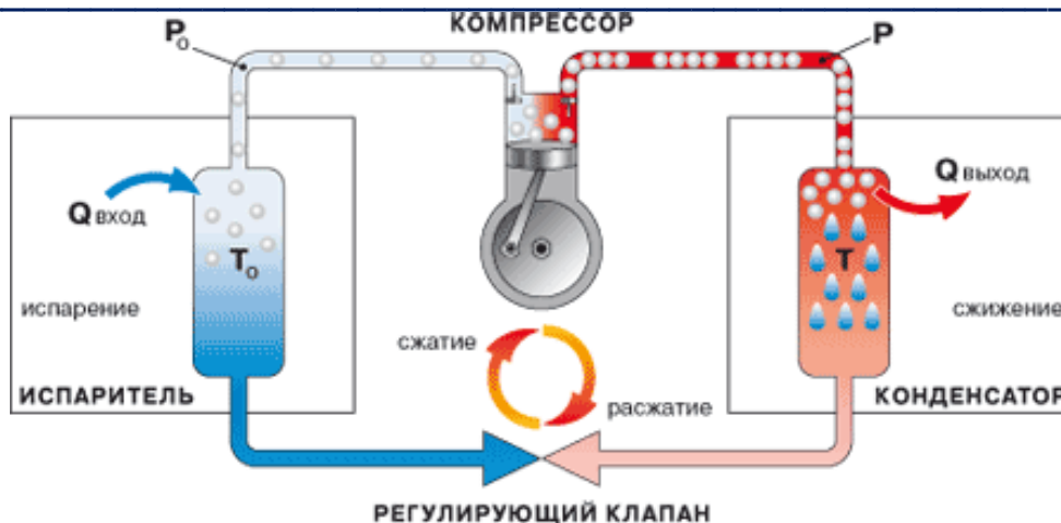
Fig. 3. Heat pump devices.
