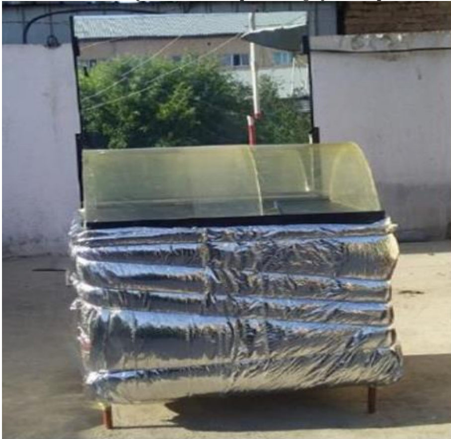
Fig.10. Experimental solar installation for the thermal processing of municipal solid waste.
