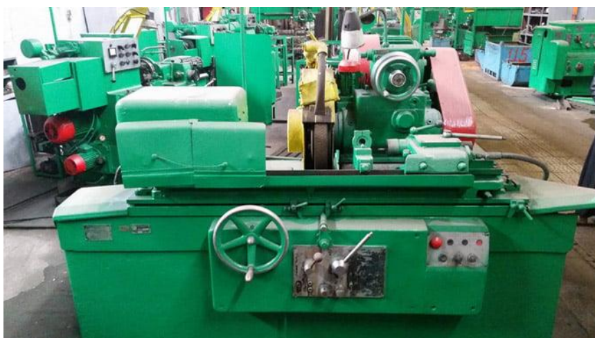
13.5-rasm. Doiraviy jilvirlash stanogi
