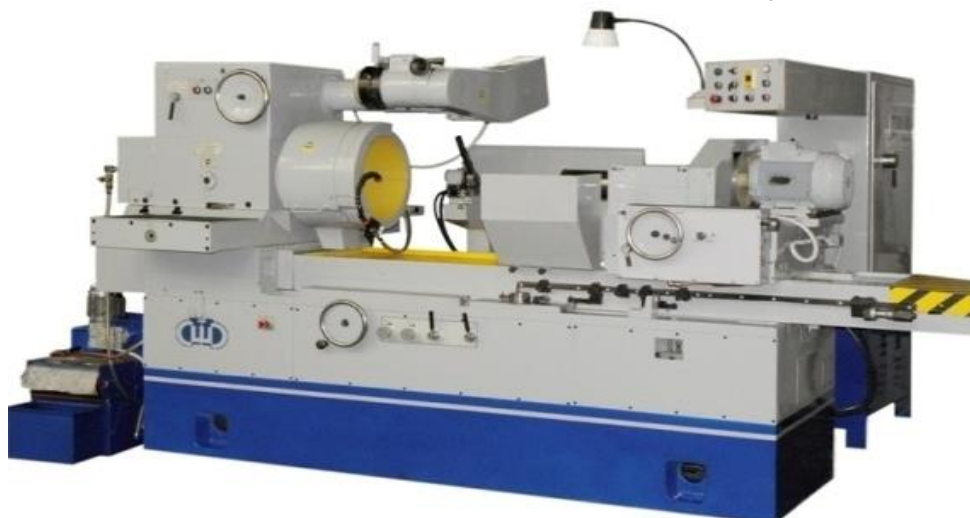
13.4-rasm. Doiraviy jilvirlash stanogi
