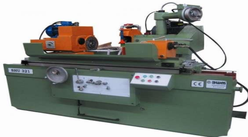
13.3-rasm. SHU-321 tipli jilvirlash stanogi
