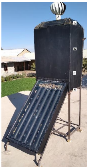
Fig.1. Natural image of a solar dryer:
