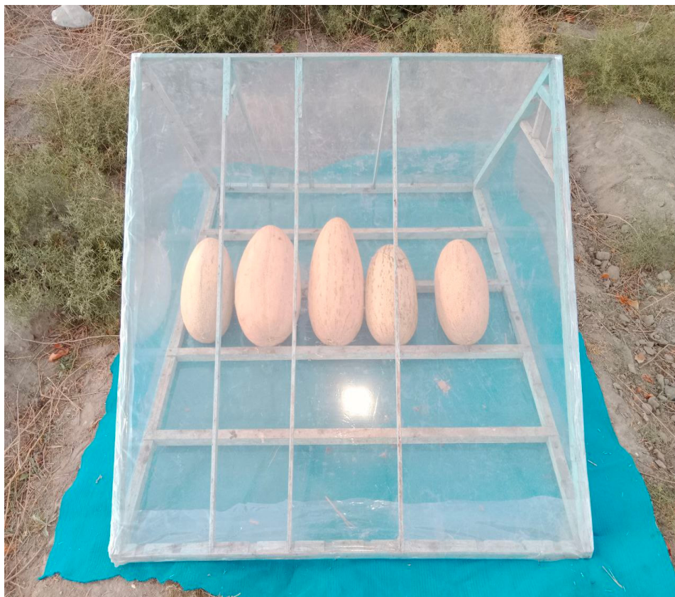
Figure 2. Greenhouse Solar Unit for Preliminary Melon Treatment.
