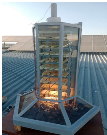
Figure 5. Real-life Image of the Solar-Infrared Drying Unit Operating on Infrared Radiation
