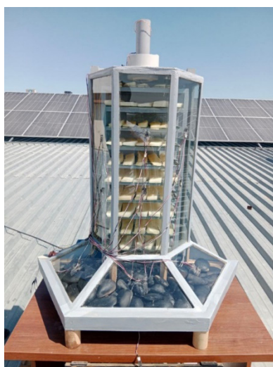
Figure 4. Real-life Image of the Solar-Infrared Drying Unit Operating on Solar Radiation
