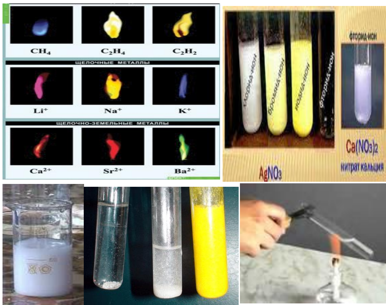
33-rasm. Metallar yonganda olov Sifat reaksiyasida cho'kma rangining hosil rangining o'zgarishi bo'lishi
