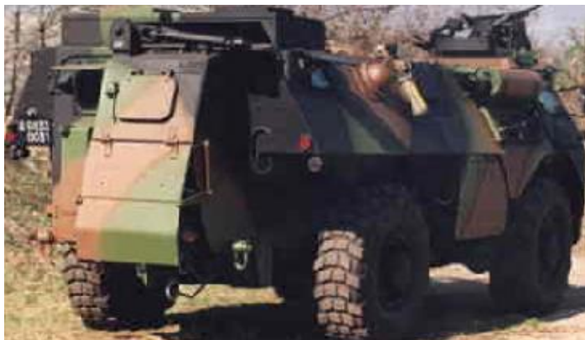
41- Rasm. VAB RECO NBC rusumli radiatsion, kimyoviy biologik razvedka mashinasi
