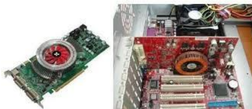
5.6-Rasm. Video adapter va uning bosh plataga ulanishi
