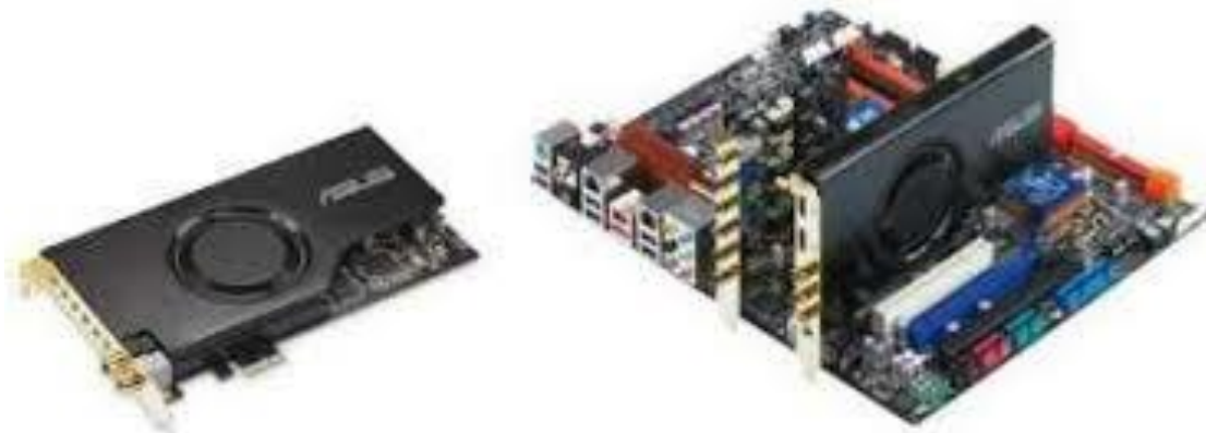
5.5-Rasm. Audio adapter va uning bosh plataga ulanishi
