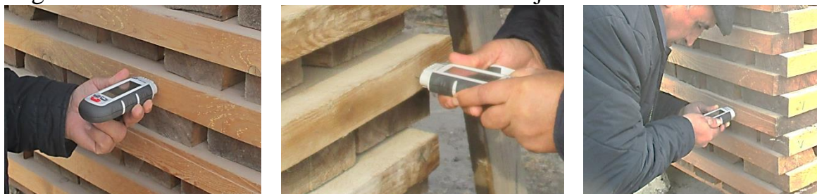
2-rasm. GEM namlik o'lchagich bilan yog'och (taxtalar) namligini o'rganish jarayoni
