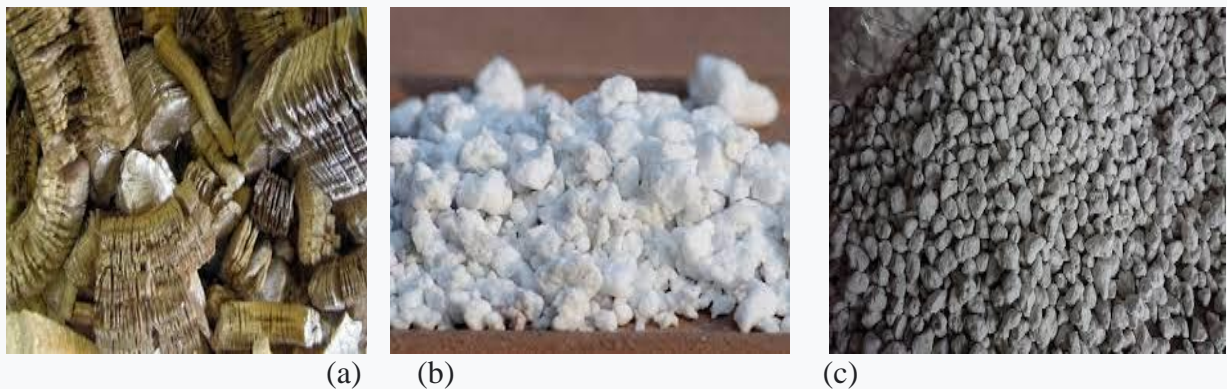
Figure 1. expanded vermiculite(a), pelite(b), pumice(c)
