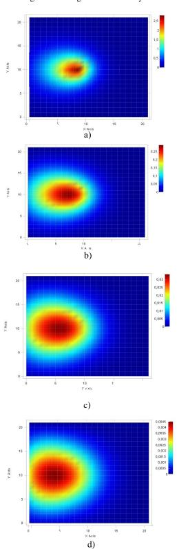
**Figure 2**. Visualization of the processes of transfer and diffusion of harmful substance - nitric oxide - in the atmosphere: a) z = 200 m; b) z = 300 m; c) z = 400 m; d) z = 500 m.
