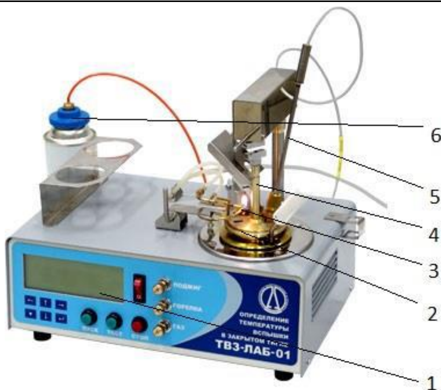
6-rasm. "TB3-ЛАБ-01" asbobini o'rnatish sxemasi: 1- boshqaruv pulti, 2-tigel, 3-gorelka, 4-aralashtirish moslamasi, 5-termopara, 6-gaz balloni.
