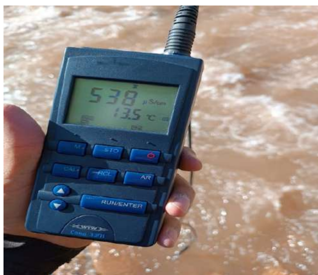
Figure 1. The process of determining water elector conductivity using a conductometer.
