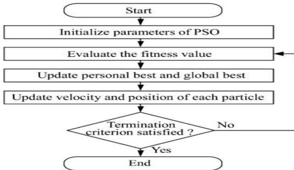
Figure 2. Flow chart of Particle Optimization
