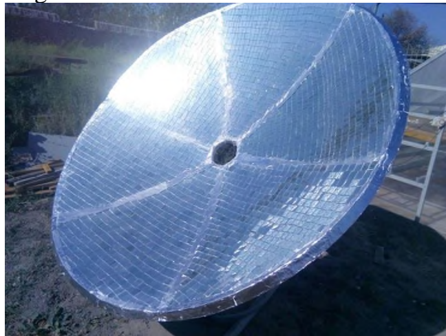
Fig.2 Appearance of the fabricated parabolic concentrator
