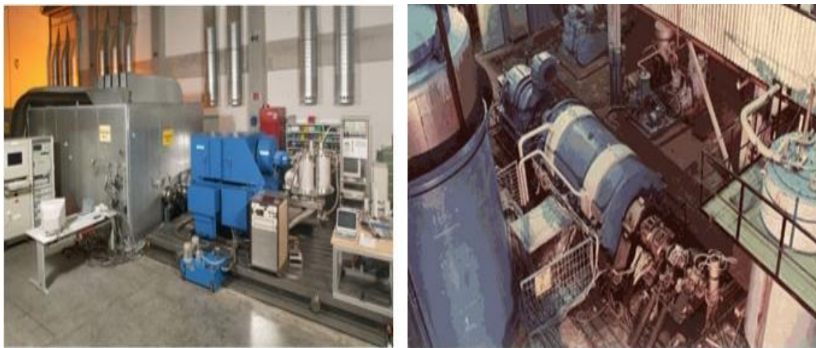
Figure-3. High-temperature superconducting generator of Siemens concern and generator developed at Elektromash Research Institute.
