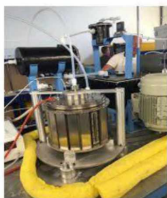
Picture-1. Electro Hydrogen Generator (EHG) and its working principle
