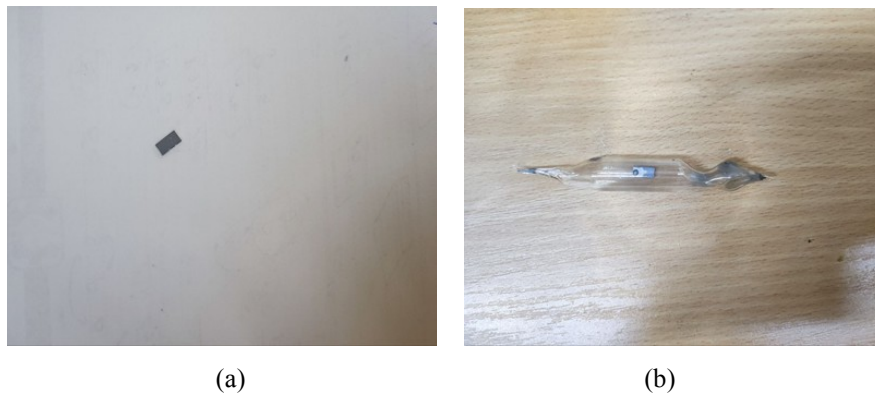
Figure 1. KDB-3 silicon sample in its initial state (a) and placed inside the ampoule (b).
