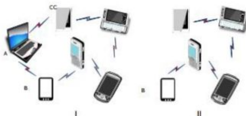
Figure 1: MANET network. I) Connection between nodes B and C in the presence of A, II) Connection between nodes B and C without the presence of A.
